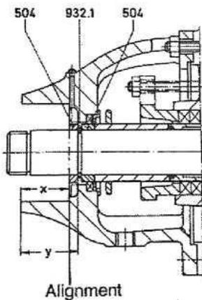
Fig. 12 correctly sized spacer ring
