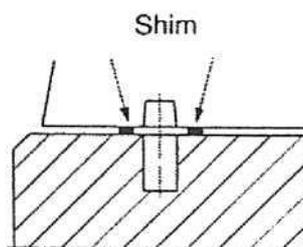
Fig. 5 Fitting shims Uniformly tighten up the bolts.
