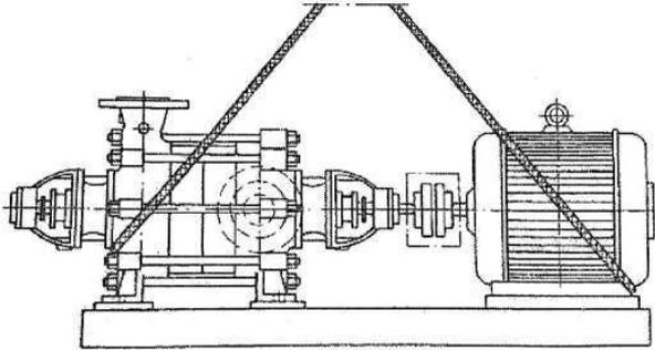
Fig. 1 Pump and motor on a common baseplate
