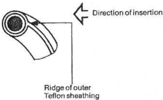
Fig.15 Teflon-sheathed O-ring
