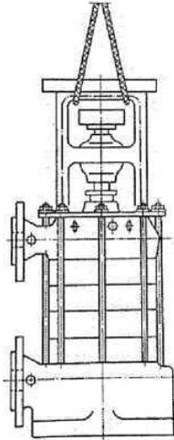
Fig. 3 Pump without motor
