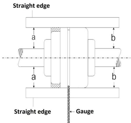
Fig.6 aligning a non-spacer type flexible coupling
