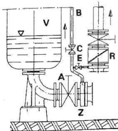
Fig. 8 Suction line and vacuum balance line
