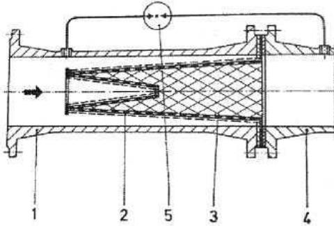
Fig. 7 Conical strainer for suction line
